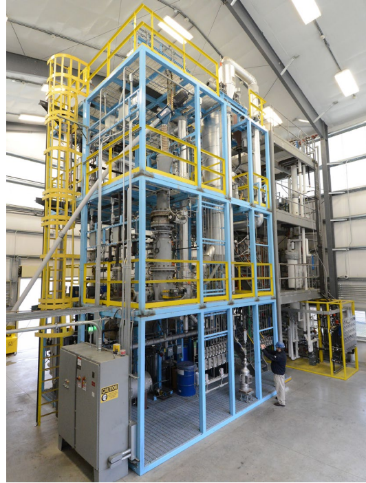
Pilot unit for biomass conversion to biofuels in RTI's Energy Technology Development Facility in Research Triangle Park, NC
