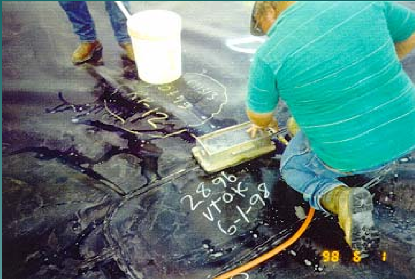
Seam Testing - Vacuum
