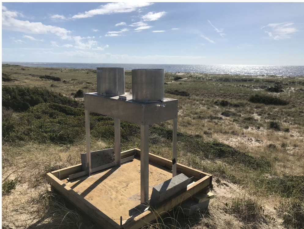
Figure 3: Remote wet/dry deposition sampling station at Baldhead Island located on a 50 ft. dune ridge overlooking Cape Fear. This will allow collection of both wet and dry deposition samples representing a true marine air mass during certain wind directions.
