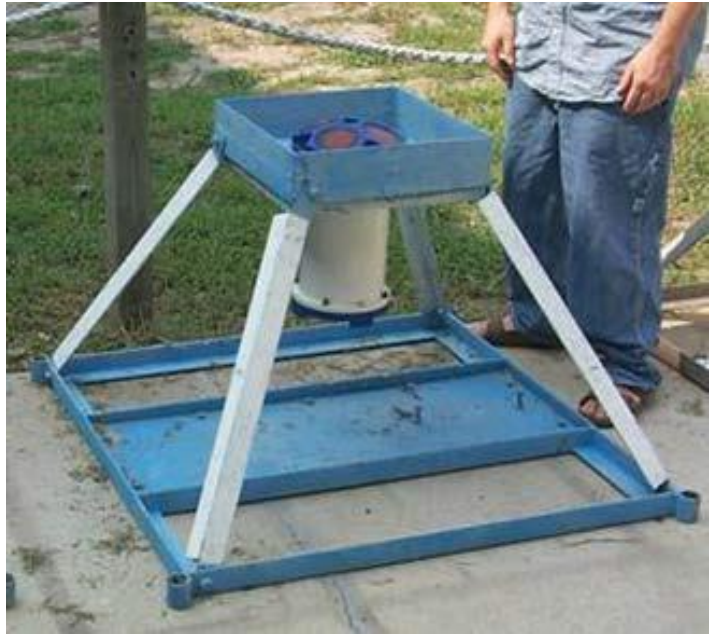
Figure 5. Acoustic Doppler Current Profiler (ADCP) in a typical mounting stand.
