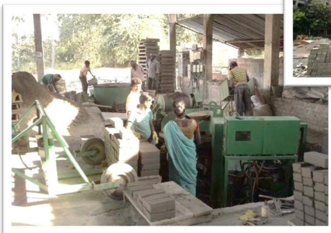
In India, within a radius of 100km from coal based thermal power plants, no person shall manufacture clay bricks, tiles or blocks (for use in construction activities) without mixing at least 25 percent of ash with soil on weight basis. (Ecobrick.in)
