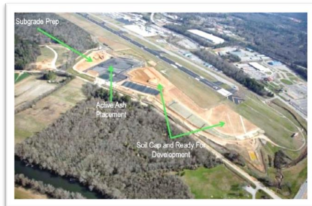
Fully-lined engineered structural fill at Asheville Airport (Charah)
