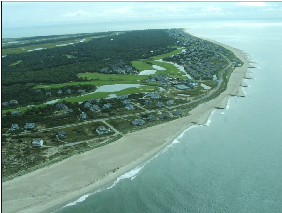
Figure 9. Groin field installed in 2005 at Village of Bald Head Island. Photo: NCDCM, 2007
