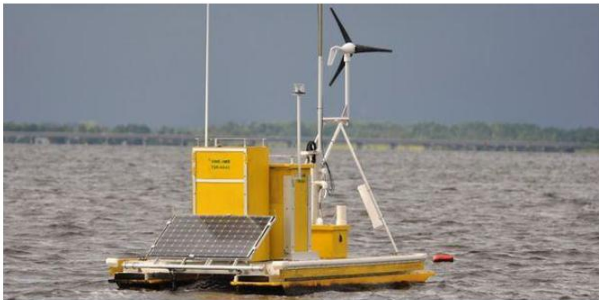
Figure 3. Autonomous Vertical Profiler (AVP)
