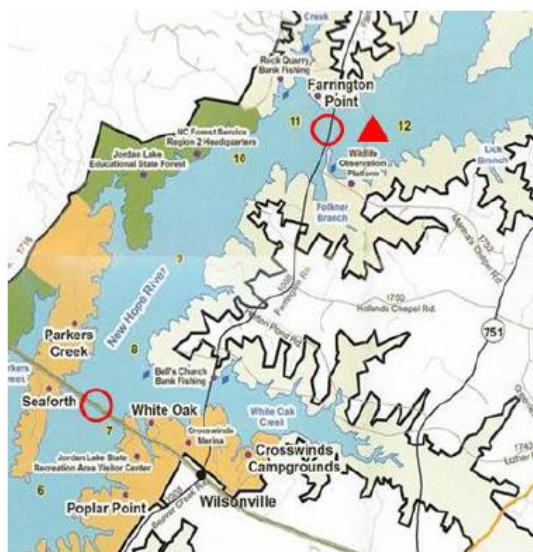
Figure 2b. Locations of ADCPs and thermistor string (circles) and the nutrient limitation bioassays (NC DEQ DWR station CFR086F) in the New Hope Creek arm of Jordan Lake.
