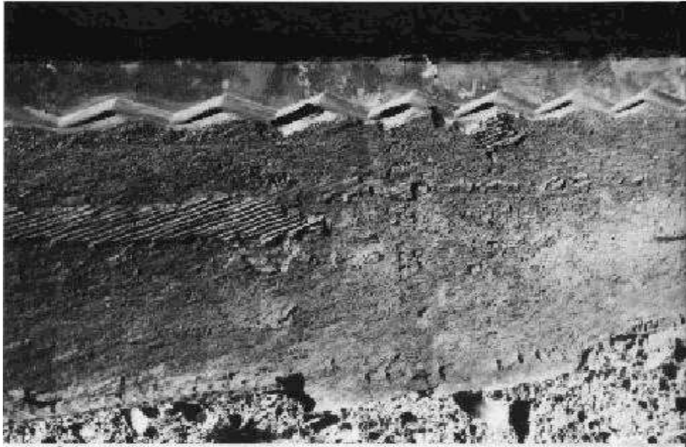
Figure 32 shows a retread bond failure. The tread rubber has separated cleanly from the casing, without wire ply belts. The rough surface patches indicate a rubber-to-rubber separation.
