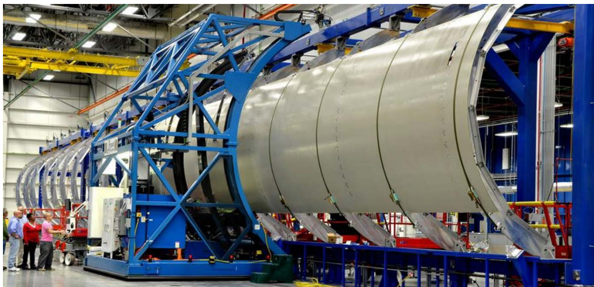
Figure 7: Aircraft Fuselage Manufacturing by Spirit AeroSystems at Their Existing NCGTP Facility
