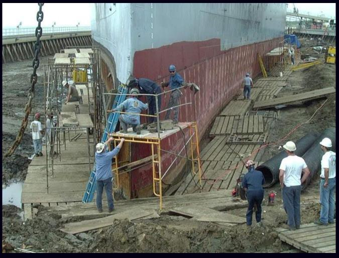
STEEL HULL PLATING REPAIRS
