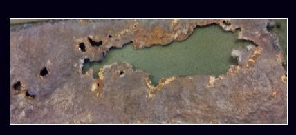
SECTION OF STARBOARD STEEL HULL
