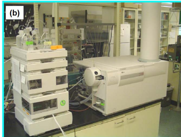
Figure 2. Picture of the (a) UPLC/MS/MS and (b) LC/TOFMS systems used
