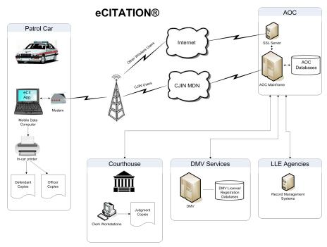
eCITATION® was developed using n-tiered architecture. The applications are either PC based or hosted on the NCAOC Websphere application server. The various components utilize the following languages: Visual Basic 6.0, JAVA Server Pages (JSP), COBOL, CICS, and HTML. Data is stored in an MS Access database on the PC and in DB2 and IMS tables on a Z-OS platform. eCITATION® interfaces with other NCAOC systems, local law enforcement records systems, and NCDMV.
