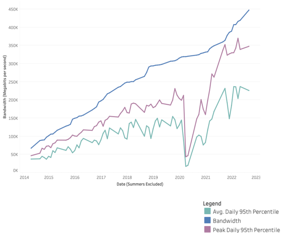
Figure 3: Statewide Contracted Bandwidth, Peak, and Average Utilization for all PSUs using NCREN.
