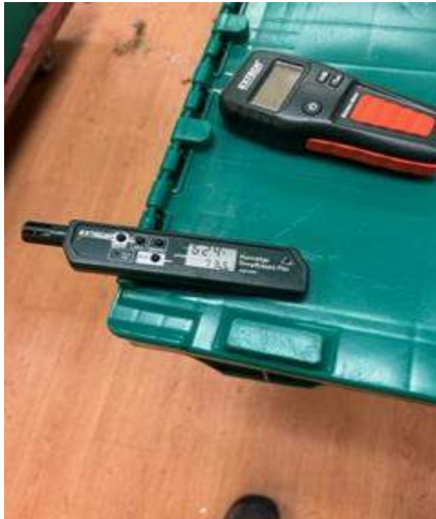
Elevated relative humidity levels measured in the conference room. Elevated relative humidity levels were measured throughout the facility.
