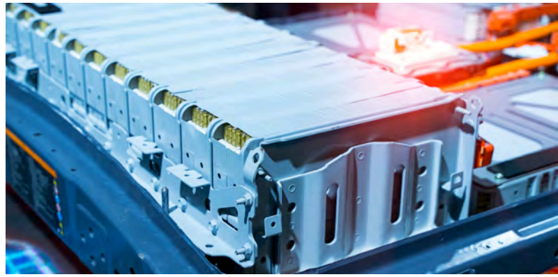
Electric car lithium battery pack and power connections.
