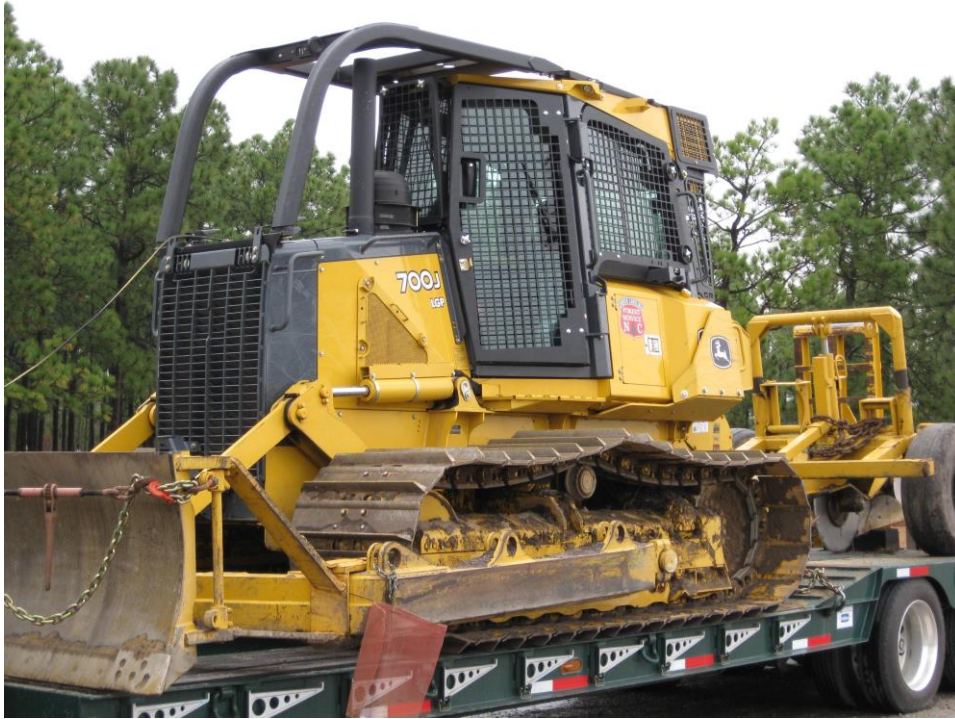
Figure 8. This John Deere 700J is one of the 93 wildland fire tractor plow units across the state.
